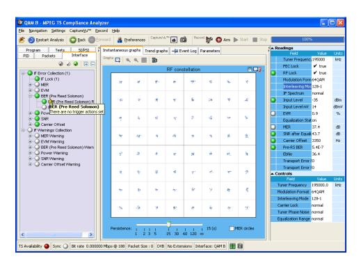
Figure 44: Interface view - RF - QAM (Annex B)
