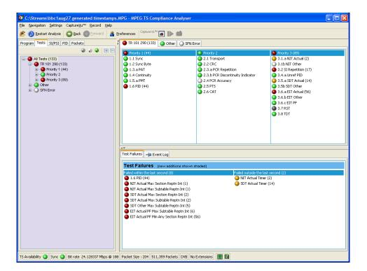
Test grouping differs between digital video standards. However, all of the currently implemented standards contain a subset of the relevant TR 101 290 tests. Note that in standards other than DVB, the tests are not numbered.
