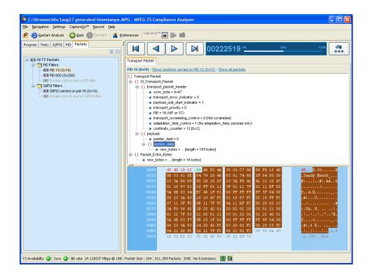
The packet transport header bytes are displayed in red. Similarly, bytes greater than 188 are displayed in gray. The adaptation field, where present, is displayed in blue.
