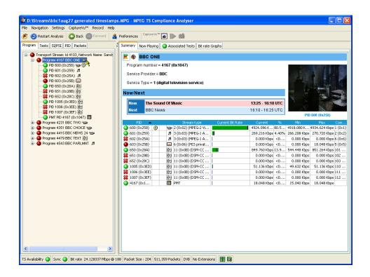
Figure 83: Program PID bit rate - bar chart
