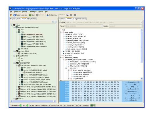
The table pane shows all fields that make up a section (for example, PMT). The fields are arranged in a hierarchical order. The presence of subordinate fields is indicated using  $\{ \}$  bracket symbols adjacent to the container field. The container can be expanded or collapsed by clicking the + or – icon.
