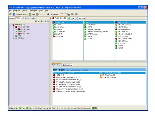
Figure 30: Tests Navigation view
