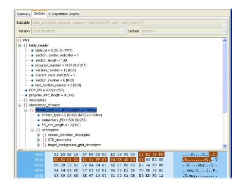
Figure 36: Section payload
