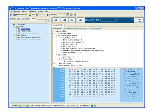
The packet navigation view shows a tree structure which represents the packets within a stream grouped according to content, including PID value, SFN mega-initialization packets (MIPs) (DVB only), and ISDB-T information packets (IIPs).
