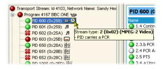
An LED associated with each elementary stream node indicates the status of the tests relating to the elementary stream.
